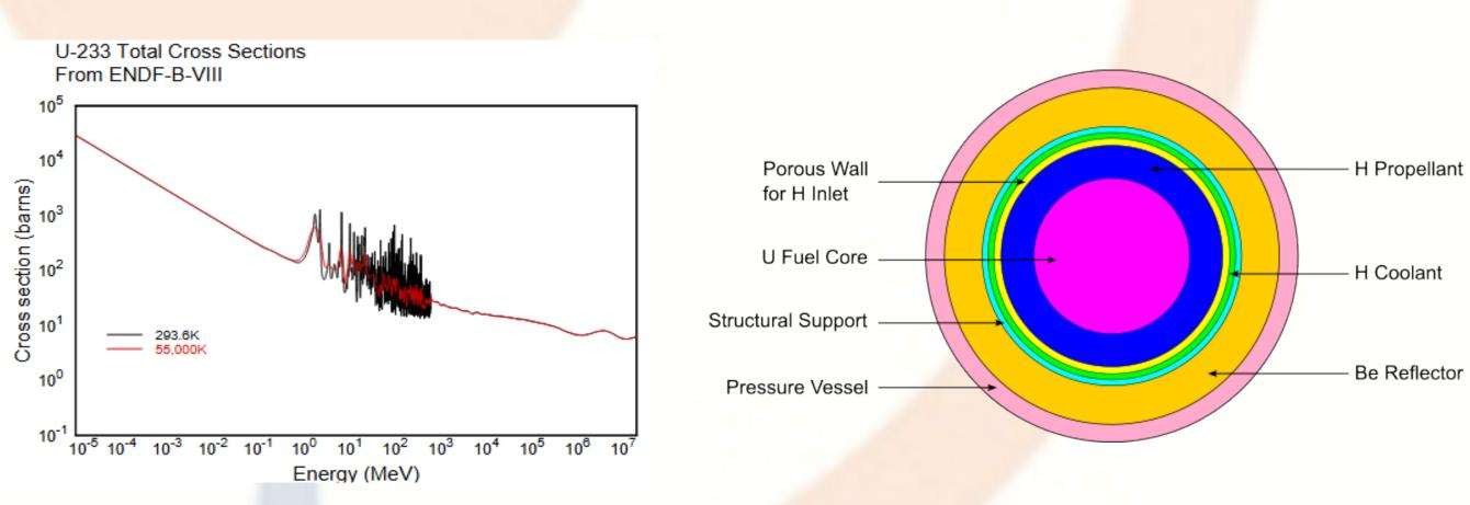
Nuclear data processing code NJOY21 is used to generate the various crosssection ACE libraries for all GCR model materials at temperatures ranging from 1,200 K to 55,000 K. Monte Carlo N-Particle (MCNP) radiation transport code and OpenMC are used to generate the neutron particle tracking data and collision physics interactions inside the GCR model. Gkeyll, will be coupled with MCNP to provide an accurate heat transfer profile from the fissioning plasma to the pressure vessel.
