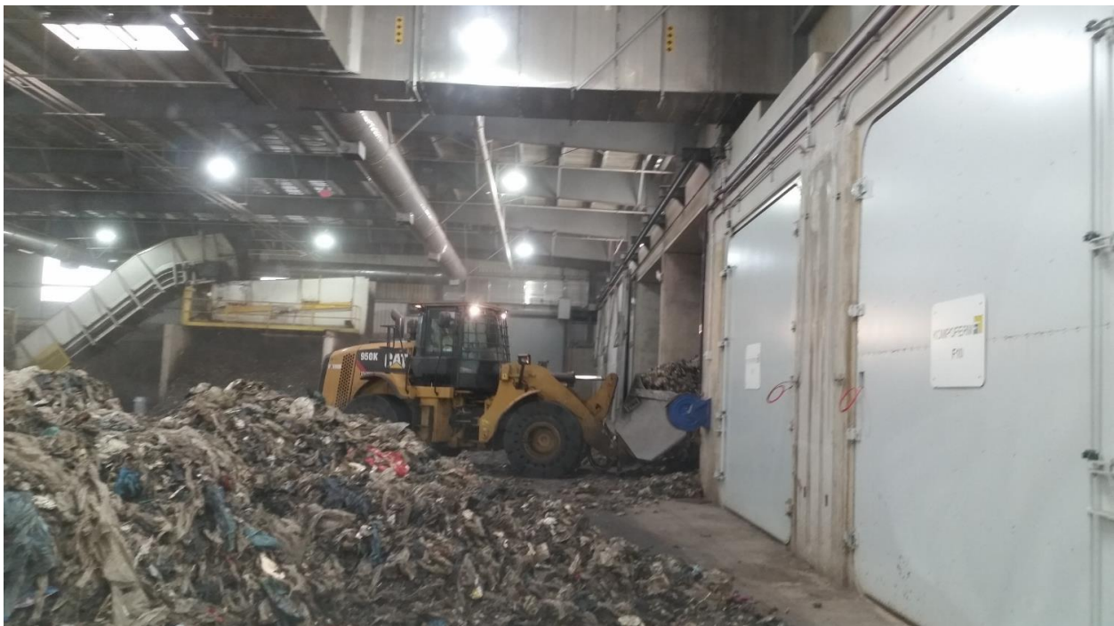
Figure 4. High Solids Anaerobic Digestions System for SSO in San Jose, CA
