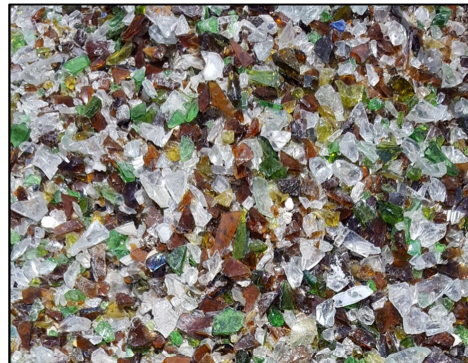
Step 2: Crush to Cullet Size, Remove Additional Contaminants
