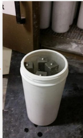
Bars submerged in alkali solution (1N NaOH) and heated at 40°C
