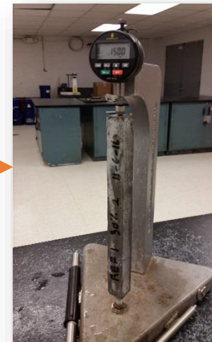
Expansion of specimens is measured over 14 days
