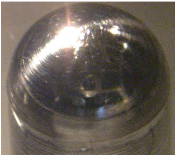
Figure 7-3: Image of the hemispherical electrode during the polarization measurement of oxygen reduction reaction.
