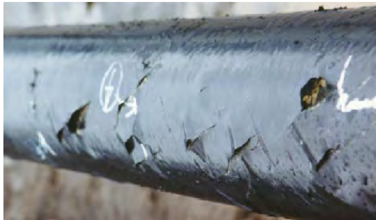
Figure 10-1: Pipe that exhibits many coating holidays. Pipe was coated in the late 60's and dug up in 1996. 2
