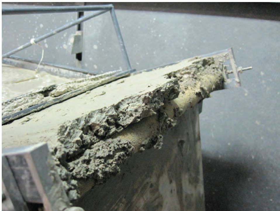
Figure 4-11. A thickened clay cake with an average solids content of 24.4 wt% was produced under the electric field of 8 V/cm. The electrodes distance was 3.2 cm and the residence time was 3.3 h (photograph by Rui Kong).
