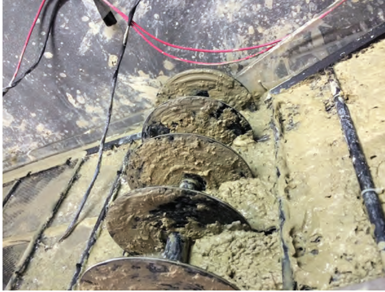
Figure 5-12. Excessive build-up of deposit in the cake formation zone caused solids dam at wheels. E=4 V/cm, \tau=3 h (photograph by Rui Kong).
