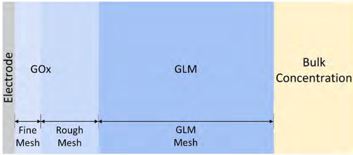
Figure 3-3. Spatial discretization of the entire glucose sensor numerical domain. Each mesh spacing consists of 200 nodes, plus an additional node for the electrode for a total of 601 nodes.
