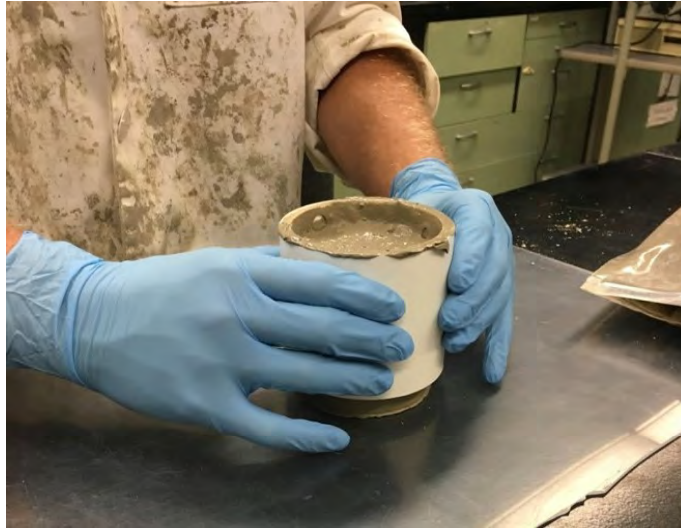
Figure 3-3. Photograph of the slump test in progress. Photograph courtesy of Jeremy Kleiman.
