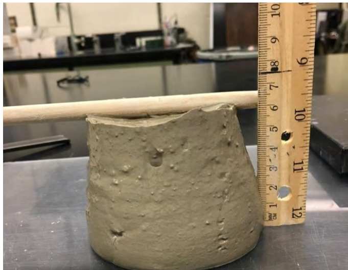
Figure 3-4. Photograph of a yielded clay sample. The slumped height of the clay sample was recorded and related to the yield strength. Photograph courtesy of Jeremy Kleiman.
