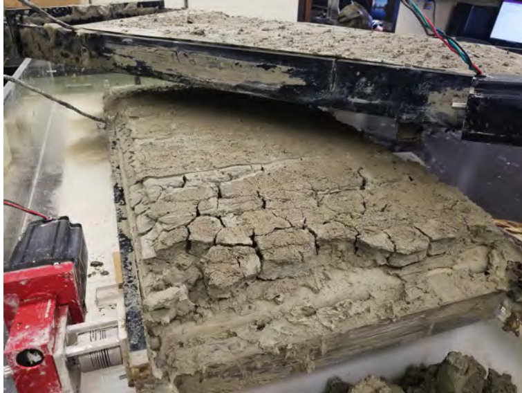
Figure 4-11. Dewatering unit from the collection side. The discharge-side electric field was 4.8 V/cm and the belt speed was 0.38 cm/min. The unit produced cake with a solids content of 36 wt.%. This image was taken from an experiment used to troubleshoot the prototype and was not used in the economic analysis. Photograph courtesy of author.
