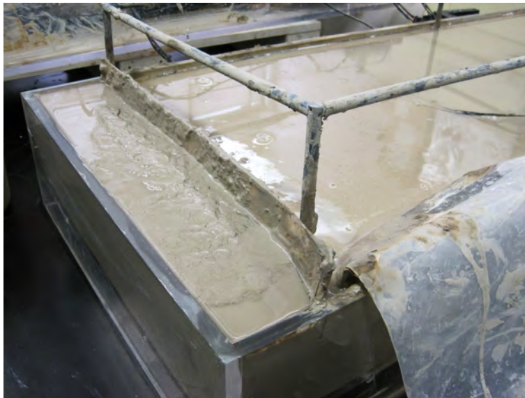
Figure 4-3. Collection area of the clay thickening unit showing an accumulation of thickened sludge produced at an electric field of 1.2 V/cm, a feed rate of 20 mL/min, and a belt speed of 1.3 cm/min. Sludge accumulated for approximately 30 minutes. Photograph courtesy of author.
