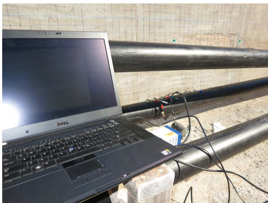
Figure 6-3. Experimental setup of the indirect impedance measurement. Photograph taken at the Texas A&M mock bridge. The Gamry Reference 600 potentiostat is the white/blue box in the center of the photograph.
