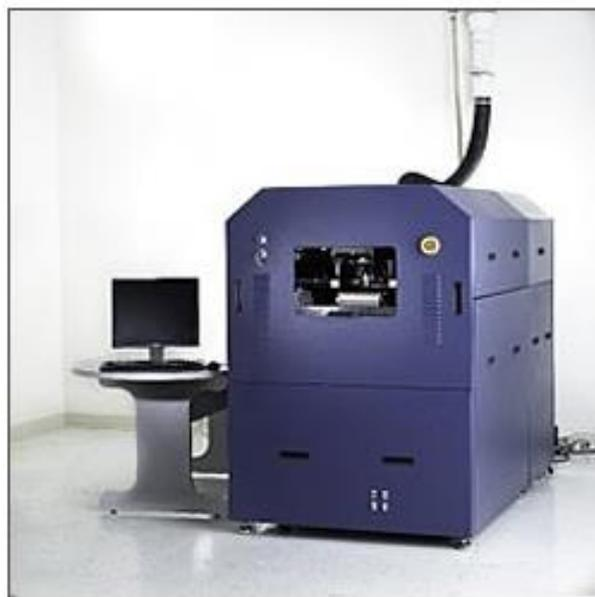
VarioEdit Laser Assisted Chemical Etching tool
