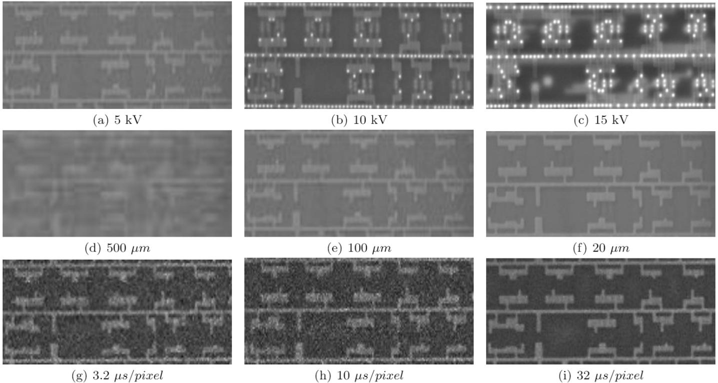
**Figure 4.** SEM images variations with different [(a), (b) and (c)] Beam voltages, [(d), (e) and (f)] Field of views and [(g), (h) and (i)] Dwelling times.
