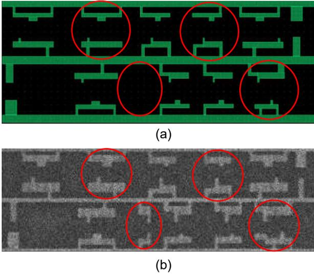
**Figure 8.** (a) Layout of the smart card chip (b) SEM image of the corresponding area. (Circled areas reflect modification or insertion of the logic cell.)
