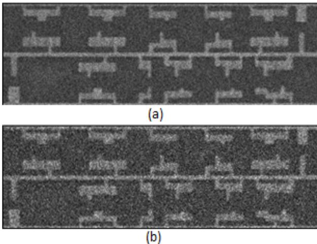
**Figure 9.** SEM images obtained by different imaging speed. (a) Speed 6:  $32 \mu\text{s}/\text{pixel}$  and (b) Speed 5:  $10 \mu\text{s}/\text{pixel}$ .
