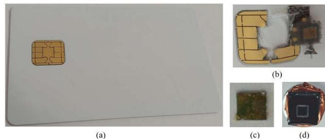
Figure 3. Sample preparation: (a) Smart card, (b) Packaged die removal, (c) Bare die and (d) Backside thinned die mounted on SEM stub.
