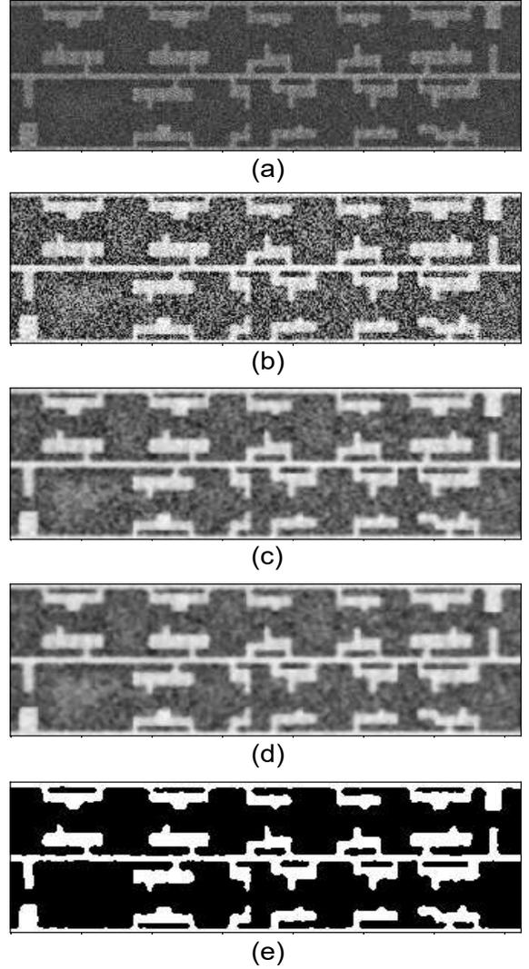
**Figure 5.** Image pre-processing. (a) Original SEM image, (b) Histogram equalization, (c) Gaussian filtering, (d) Median filtering and (e) Thresholding.
