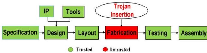
**Figure 1.** Untrusted foundry attack model.
