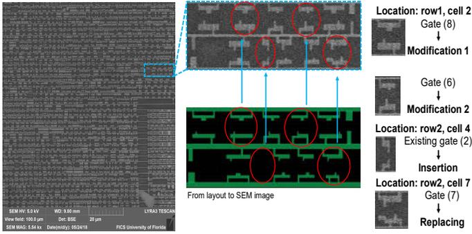
Figure 12. Layout vs. SEM image comparison results.
