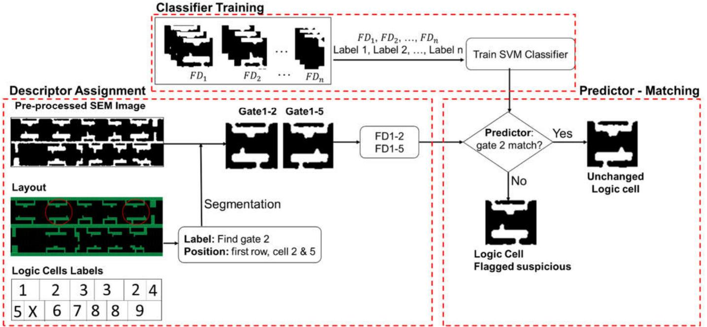
Figure 6. Trojan Scanner matching engine.
