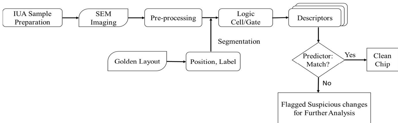
Figure 2. Trojan Scanner 2.0 process flow.
