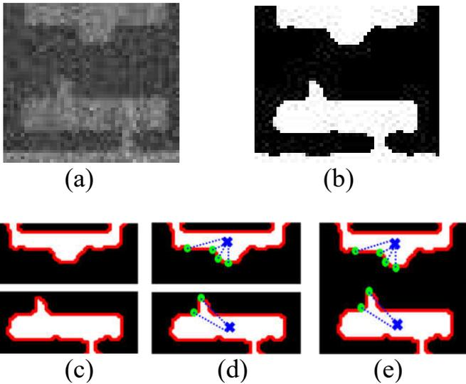
Figure 7. Generation of Fourier descriptors. (a) Segmented SEM image of a logic cell, (b) Binarized image of logic cell, (c) Converting logic cell into closed shape, (d) Generating Fourier descriptor for upper and lower closed shape. (e) Combining upper and lower descriptors for whole logic cell.
