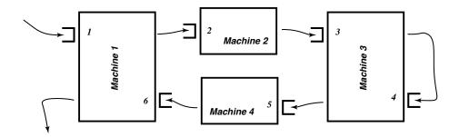
Figure 6. A re-entrant line with regulation.
