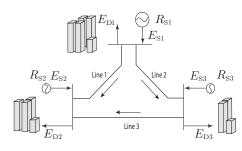
Fig. 2. Texas model: a simplified 3-bus network.
