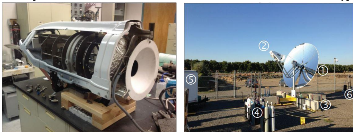
Figure 6. On the left is the STARS solar methane reforming reactor with the aperture for sunlight on its right hand side. On the right is the STARS systems mounted to a tracking parabolic concentrator for prototype testing. 28
