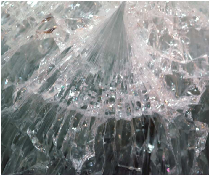
Fig. 3 Crack fans that separate regions of bundled radial cracks and unbundled radial cracks.
