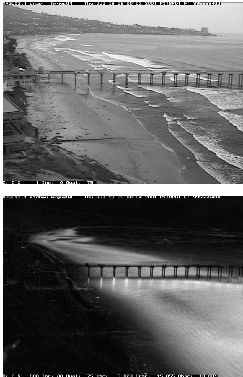
Figure 1. Images from a CIL Argus camera, looking south towards the study site located 400 m south of SIO pier, on 19 July 2001 (later referred to as Case 1). (top) Snapshot. (bottom) Time lapse pixel variance, where bright regions are areas of persistent wave breaking, dark regions are areas of relatively quiescent water or land (R. Holman, personal communication).
