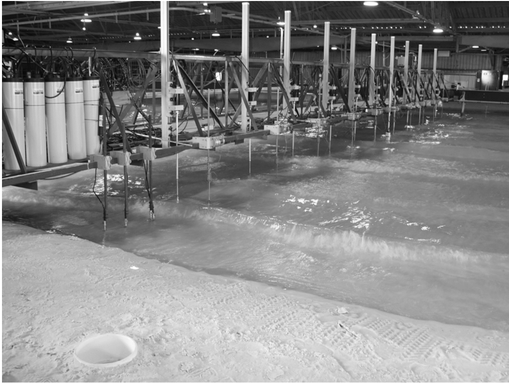
Figure 5-1. Snapshot of the Large-scale Sediment Transport Facility showing the instrumentation bridge, in situ sensors and surf zone waves.
