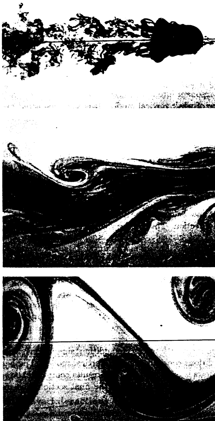
Fig.1. Wake collapse of a towed sphere in a continuously stratified fluid (from Hopfinger, 1987).
