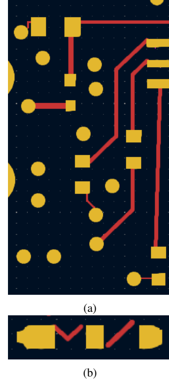
Fig. 6: (a) Good and (b) bad trace reconstructions for layer 1 of the test board.
