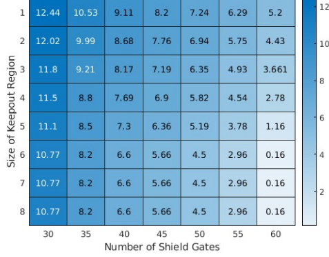
Fig. 7: Effect of keepout region and number of shield gates on the exposed area.
