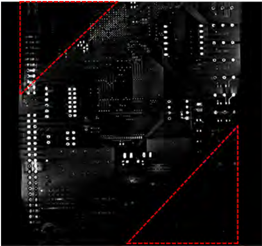
Fig. 30. Misaligned Xilinx Spartan board X-Ray CT slice
