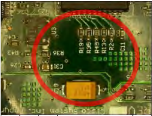
Fig. 17. Optically imaged PCB section highlighting illuminance non-uniformity
