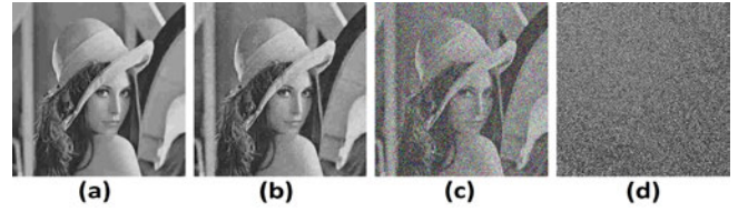
Fig. 6: Outputs for the obfuscated 2D-DCT with key error percentage set at (a) 1%, (b) 10%, (c) 12%, and (d) 20%. The quality drops off steeply after 10% error.
