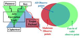
Figure 8: Overview of our proposed intersect analysis. The blue region represents the all observe point where an Asset can propagate to and the green region represents all the fanin elements of valid observe points (Ciphertext output port). The red dotted region represents the malicious observe points (Type II Trojan).
