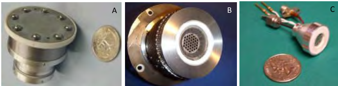
Figure 2-11. Gridded ion microthrusters. A) JPL Miniature Xenon Ion Thruster (MiXI). B) University of Giessen \mu NRIT-2.5 Miniature Ion Thruster. C) Penn State University MRIT Micro-Ion Thruster (Mueller, Hofer, & Ziemer, 2010).
