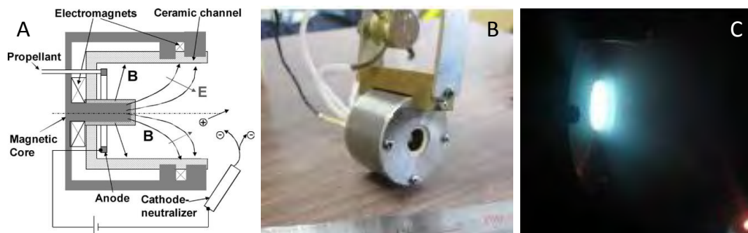
Figure 2-13. Cylindrical Hall effect microthruster. A) Schematic (Polzin, Raites, Gayoso, & Fisch, 2010). B) Prototype 7 mm channel cylindrical thruster. C) Prototype thruster in operation (Ikeda, Togawa, Nishida, Tahara, & Watanabe, 2011).
