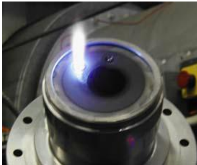
Figure 2-2. Plasma igniter in operation [12]
