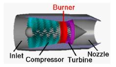
This is an annular tube, or ring of tubes, made from heat-resistant steel, in which the fuel and air are mixed and ignited. It is designed to achieve the most efficient combustion of the mixture so that the maximum possible heat energy is extracted from the fuel to give the greatest rise in temperature and hence expansion of gases.
