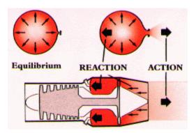
The section of the gas turbine in which combustion takes place, known as the "hot end," operates in the same way as the balloon. The reaction to the gas stream that is ejected from the nozzle is felt on the parts of the engine opposite the nozzle, mainly the front of the combustion chamber and the tail cone. This force, termed thrust, it then transmitted from the engine casing to
