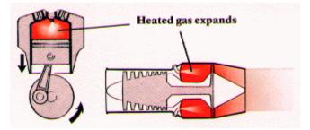
In the gas turbine, the burning is continuous and the expanding gas is ejected from the engine as an action. Using the principle expounded by Sir Isaac Newton in the 17th century - to every action there is an equal and opposite reaction - this action creates a reaction of equivalent force.
