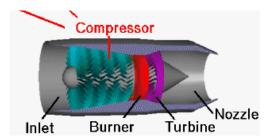
Situated at the front of the engine, the compressor draws air in, pressurizes it, then delivers it into the combustion chamber. There are two types of compressor design, centrifugal and axial flow.
