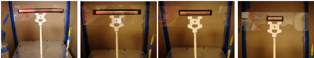
Figure 8. Experimental setup showing the four different electrode lengths tested; From left to right: 20, 15, 10 and 5 cm long actuators (0.5 cm wide, zero gap).
