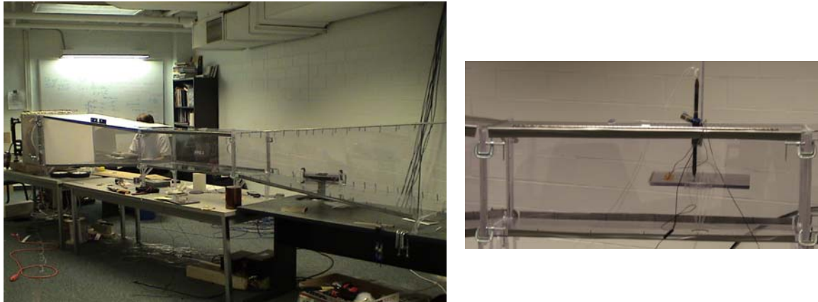
Fig. 1: CPDL experimental facility wind tunnel (left) and the setup of the test section (right).
